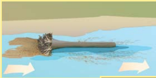
Figure 4 - Sedimentation and scouring around a LWD structure
