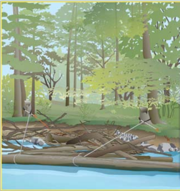
Figure 52 - LWD may be cabled to secured objects on the bank (Palmiter Method). Secure cables to downed or dead wood only
